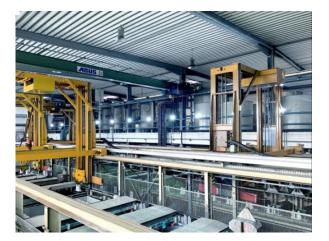
Existing systems are converted into an electroplating system for fully automated electrode coating. © Sunfire GmbH
