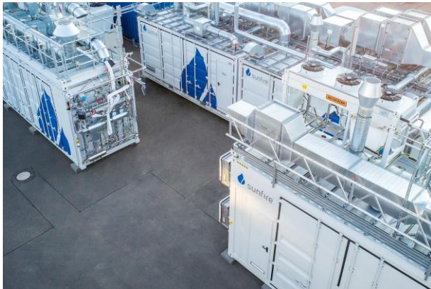
High temperature, solid oxide cell electrolyzers produced at Sunfire's headquarters in Dresden, Germany © Sunfire GmbH
